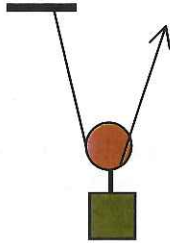
A single movable pulley MA = 2
